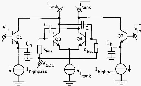
Figure 5. One section of the I/Q LC oscillator with high-pass coupling.
