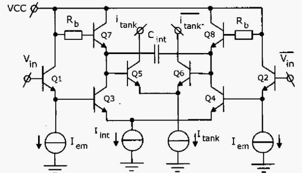
Figure 4. One section of the I/Q LC oscillator with integrators.
