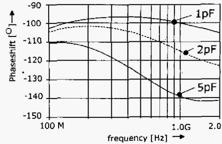
Figure 6. Simulated phase shift of  $i_{tank}(j\omega)/V_{in}(j\omega)$  for three values of  $C_h$ .
