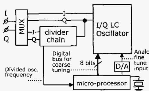
Figure 1. Wide range I/Q signal generation architecture.
