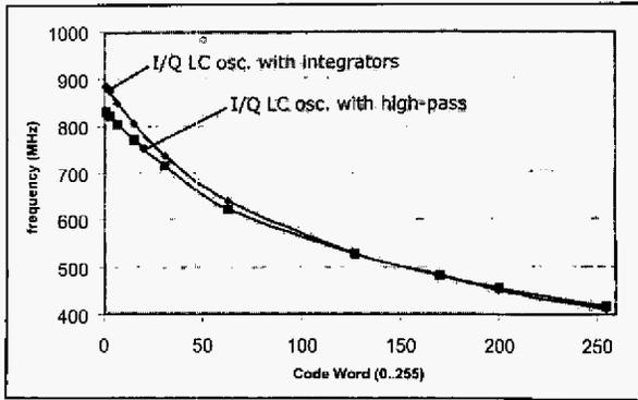
Figure 8. Frequency versus code word of both oscillators, with varactor voltage  $V_{tune}=1V$ .
