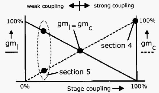
Figure 3. The ratio between  $gm_l$  and  $gm_c$  determines the strength of the coupling between two single-phase LC oscillators.
