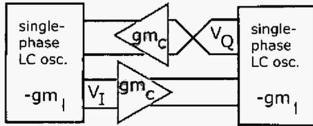
Figure 2. Block diagram of an I/Q LC oscillator coupled with transconductances  $gm_c$ .
