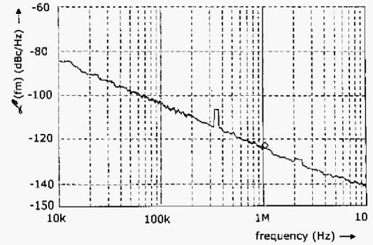
Figure 9.  $\mathcal{L}(f_m)$  of the oscillator with high-pass coupling at 417 MHz, measured with a R&S FSIQ
