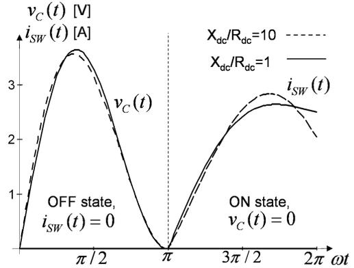
Figure 4: The switch voltage and current waveforms.
