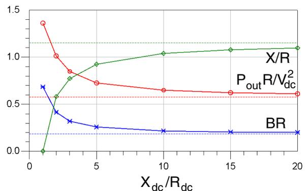
Figure 2: Effect of the finite DC-feed inductance on the Class-E circuit elements.
