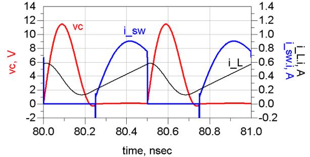
Figure 6: The switch voltage and current waveforms and the DC-feed inductance current.
