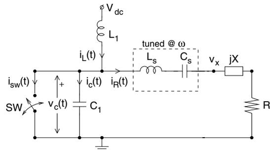
Figure 1: Class-E PA circuit.
