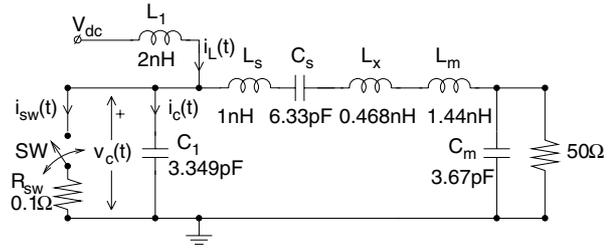
Figure 5: The Class-E PA for 2 GHz.
