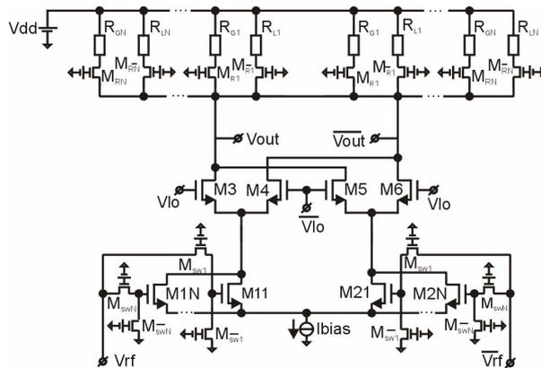
**Figure 4:** A Gilbert cell mixer with a discretely adjustable performance
