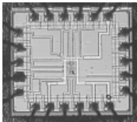
**Figure 7:** Die micrograph of the adjustable Gilbert cell
