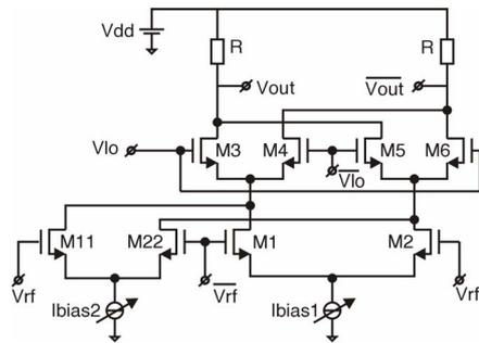
**Figure 5:** A Gilbert cell mixer with a continuously adjustable performance space
