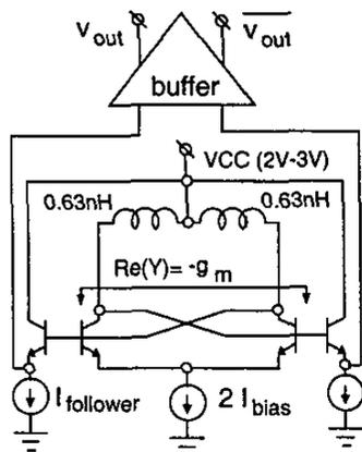
Figure 3. Circuit diagram of the varactorless 10 GHz technology demonstrator: a LC oscillator, with a 50Ω output buffer.
