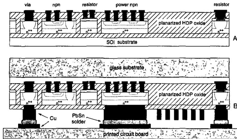
Figure 2. Illustration of the surface mounted RF IC technology.
