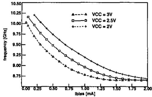
Figure 5. Oscillation frequency versus  $I_{bias}$  for VCC is 2V, 2.5V and 3V.
