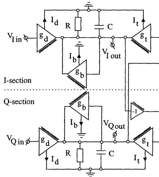
Figure 4. Behavioural model of one filter stage.
