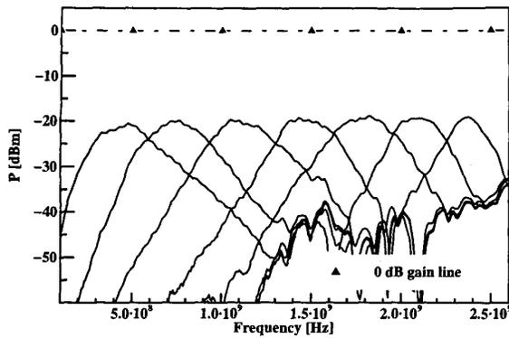
Figure 8. Measured bandpass curves for -20 dB gain setting. The high noise floor around 2 GHz is caused by the PCB and measurement equipment.
