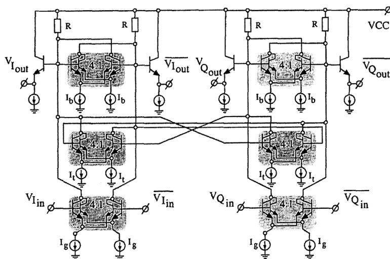
Figure 5. Simplified circuit diagram of one filter section.
