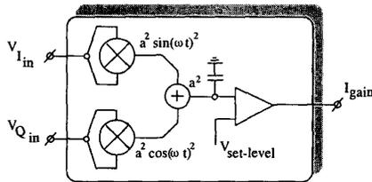
Figure 3. Block diagram of AGC control.
