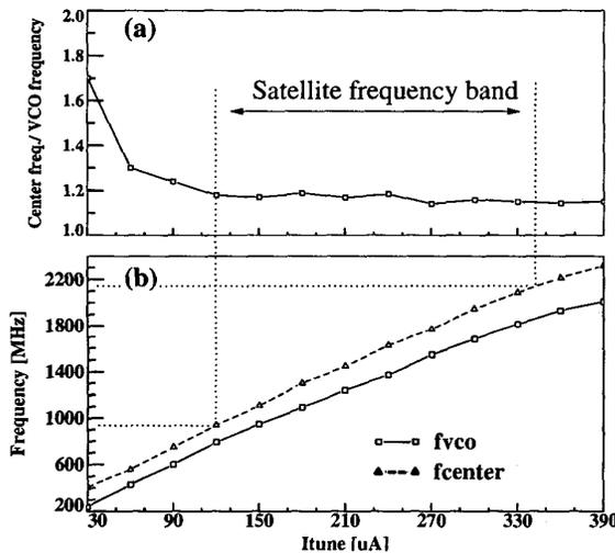
Figure 9. Measured ratio of the filter center frequency and VCO frequency versus  $I_{tune}$  (a). Frequency versus  $I_{tune}$  of the VCO and the bandpass filter (b).
