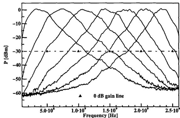
Figure 7. Measured bandpass curves for 30 dB gain setting.
