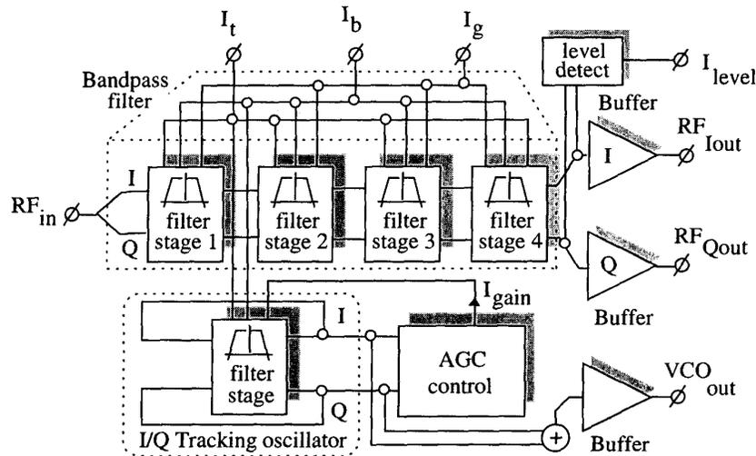
Figure 2. Block diagram of the bandpass filter with tracking oscillator.
