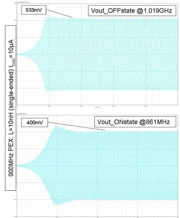
Fig. 5 Transient response for the minimum and maximum frequency in the 900MHz band when a bias current  $I_{\text{bias}}=10\mu\text{A}$  is used.
