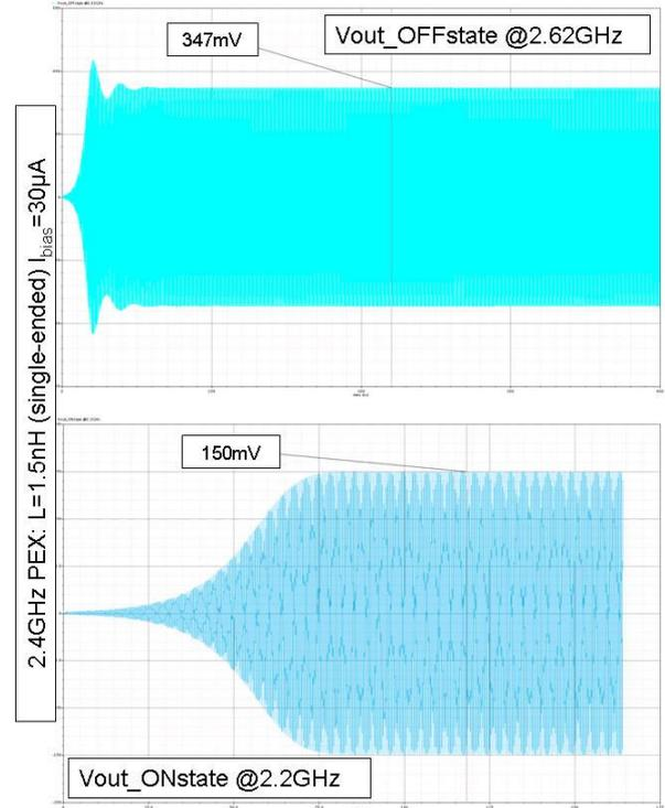
Fig.4 Transient response for the minimum and maximum frequency in the 2.4GHz band when a bias current  $I_{\text{bias}}=30\mu\text{A}$  is used.
