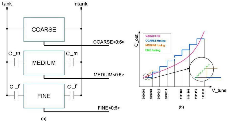
Fig. 3 Block diagram of the total capacitor bank (a) composed by the coarse, the medium, and the fine tuning banks. Discrete tuning obtained by mean coarse, medium and fine tuning is illustrated in (b).
