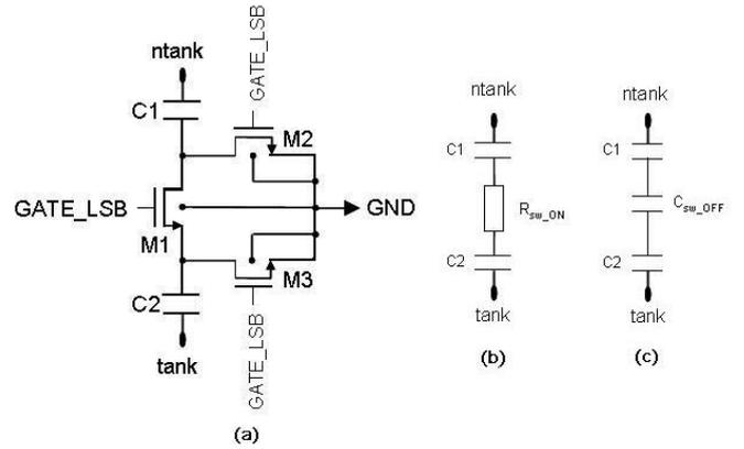
Fig. 2 Schematic diagram and on/off model of the differential switched capacitor.
