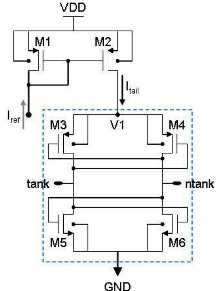
Fig. 1 Schematic view of the current source and of the complementary MOS cross-coupled pairs used as active part.
